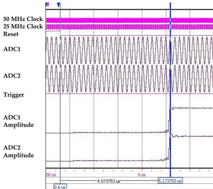
Figure 5.4: *Simulation of detector framework and arc detector core without triggering: From top to bottom the signals of the 50 MHz clock, the 25 MHz clock, the reset, the ADC1, the ADC2, the trigger, the ADC1 amplitude and the ADC2 amplitude are plotted. The blue vertical lines are indicating cursor positions for time measurement.*
