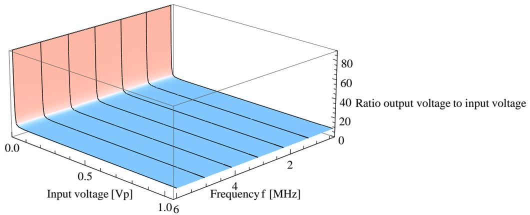
Figure A.4: *Input to output ratio of ADC2 channel: Plotted is ratio output voltage as a function of the input voltage and the frequency.*
