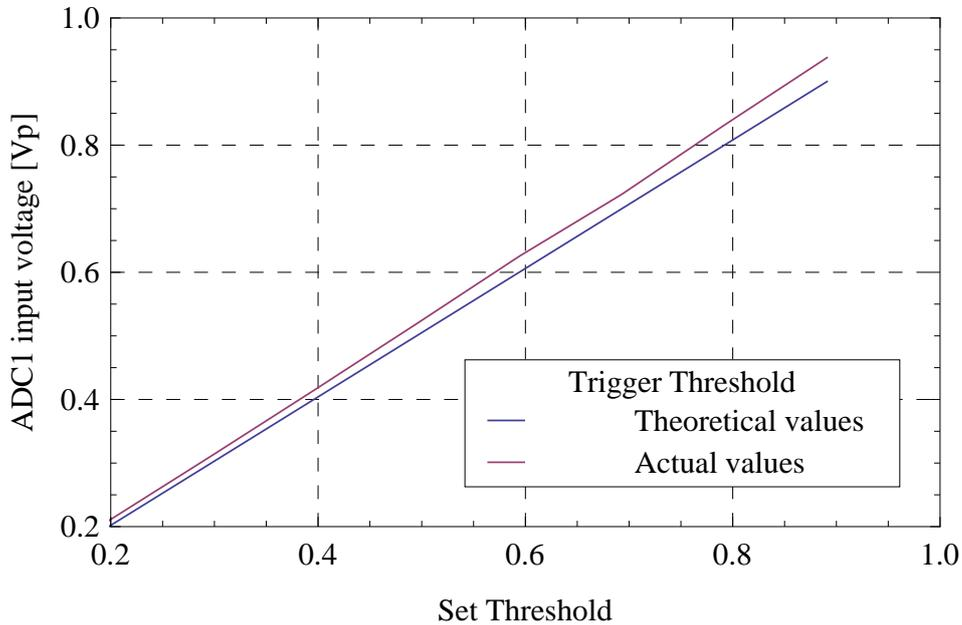
Figure 6.15: *Trigger threshold: ADC1 input voltage over theoretical and actual threshold.*
