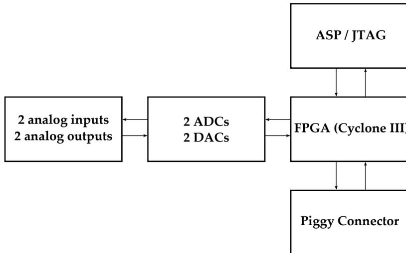
Figure 2.5: *Schematic of the FAB: The FAB provides two BNC plugs for analog input signals, which are digitized by two ADCs. The digital signals are sent to the FPGA where they are processed. Digital signals generated in the FPGA can be transformed into analog signals and can be taped over two LEMO plugs. The the piggy connector is for communication with the FIB. Programming and diagnostics of the FPGA can be done via the ASP and JTAG interfaces.*
