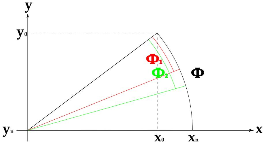
Figure 4.2: *CORDIC algorithm in rotation mode. The input vector (black) with the components  $x_0$  and  $y_0$  and an angle of  $\phi$  is rotated to align the  $x$  axis. This is done in steps of an iteration yielding vectors with an angle of  $\phi_1$  (red),  $\phi_2$  (green), and so on. After a sufficient amount of steps the vector is aligned to the  $x$  axis at which  $x_n$  represents the amplitude of the original input vector.*
