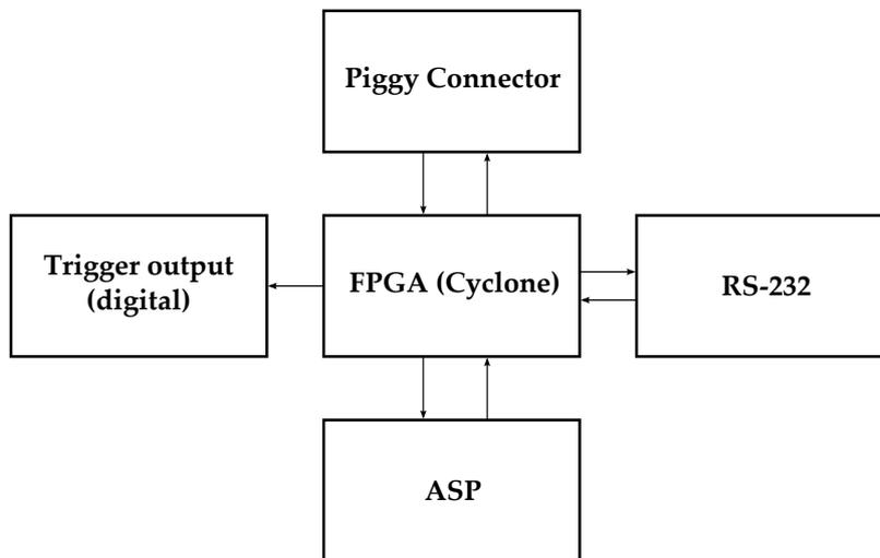
Figure 2.3: *Schematic of the FIB: The FIB provides a piggy-connector as an interface for communication with a FAB. All incoming data is processed by the FPGA. A digital trigger signal generated by the FPGA can be sent over a LEMO interface. Programming the FPGA can be done via the ASP interface. The RS-232 interface is used for communication with a PC.*
