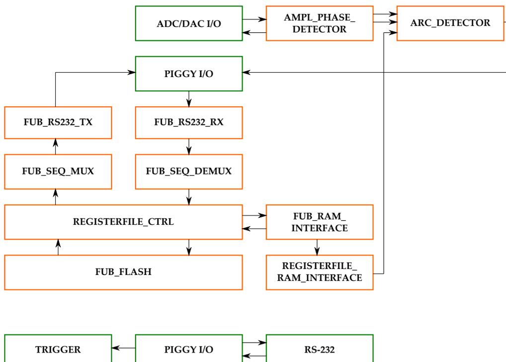
Figure 5.2: Schematic of detector framework: The upper schematic shows the principle of the program segment for the FAB, the lower one for the FIB. Ports are illustrated in green, packages in orange.
