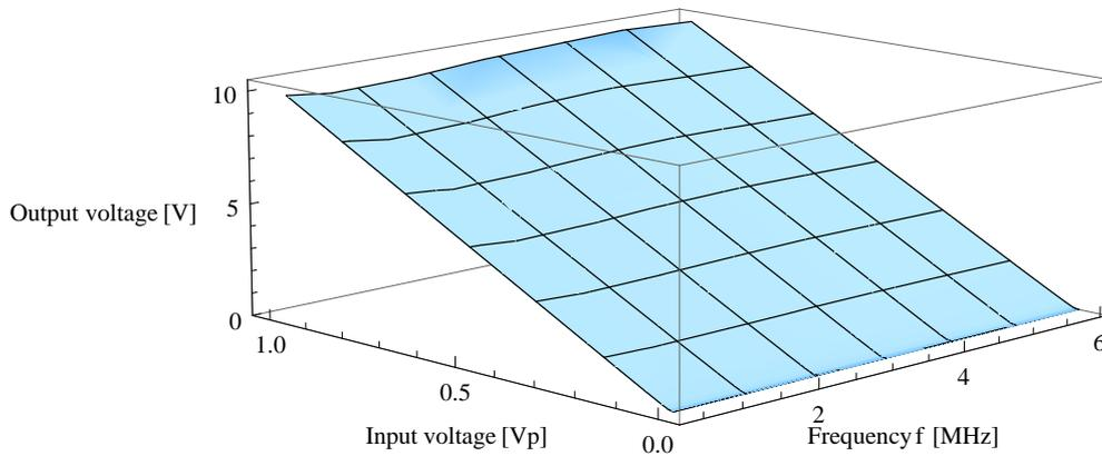
Figure 6.4: *Measured values of ADC2 channel: Plotted is the output voltage as a function of the voltage and the frequency.*
