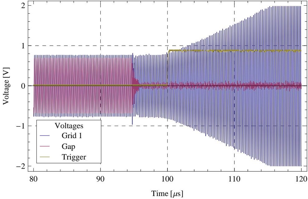
Figure 7.4: Measurement of the trigger signal of the arc detector (divided by 5 for better visibility), the grid-1 voltage, and gap voltage at a continuous wave at 3.24 MHz and a slowly rising amplitude: Plotted is the respective voltage [V] over time [s].
