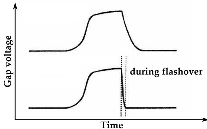
Figure 2.6: *Characteristics of the amplitude without (upper graph) and during an electric arc (lower graph). The dotted lines indicate the time interval in which the voltage drops during a flashover. [7]*
