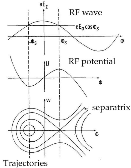
Figure 1.4: *Particle Dynamics in an RF Field: On the top the  $z$  component of the electric field of the RF wave is plotted as a function of phase. In the middle the RF potential is plotted as a function of phase. At the bottom the phase space with particle energy as a function of phase is plotted. In all three plots the location of the ideal particle is marked with the left dashed line.*
