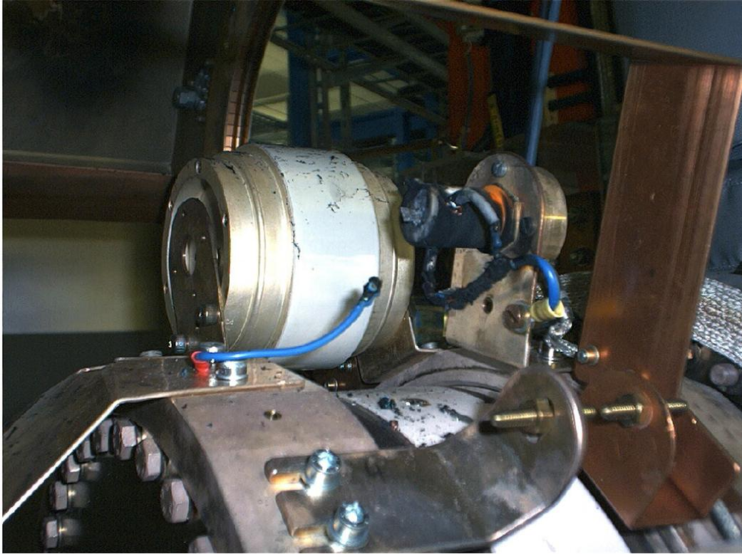
Figure 1.5: *Picture of the gap of the SIS 18 cavity after an ongoing electric arc. The arc moved due to thermodynamic effects from the predetermined point of flashover along the gap to a higher position and burned several cables.*
