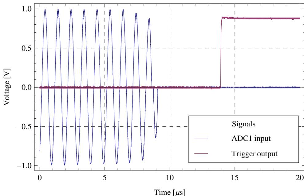
Figure 6.16: *Trigger response time: Emulated gap-voltage signal and trigger signal as a function of time. The output trigger signal has been scaled down by the factor of 5 for better visibility.*
