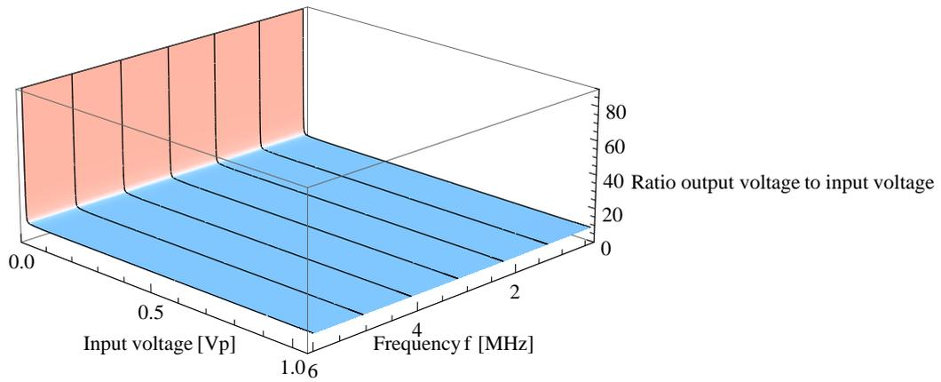
Figure A.3: *Input to output ratio of ADC1 channel: Plotted is ratio output voltage as a function of the input voltage and the frequency.*
