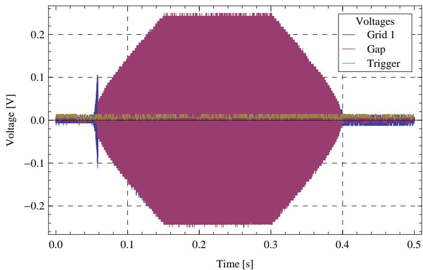
Figure 7.6: Measurement of the trigger signal (divided by 5 for better visibility), the grid-1 voltage, and the gap voltage in a realistic acceleration cycle producing no electric arc.
