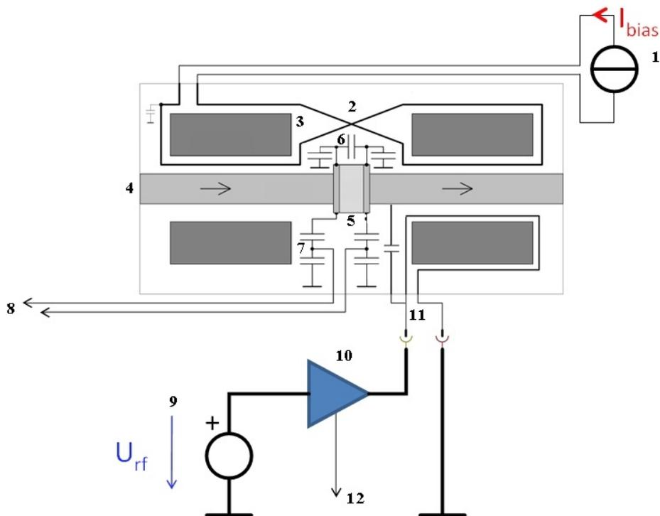
Figure 2.1: *Diagram of SIS 18 cavity including current source for bias windings (1), bias windings (2), ferrite ring cores (3), beam pipe (4), ceramic gap (5), capacitors for adjusting frequency range of the cavity (6), voltage divider (7) for gap voltage monitoring (8), voltage source (9), tetrode amplifier to power the cavity (10), mixed coupling (11) and output for monitoring grid–1 voltage of the tetrode (12). [11]*
