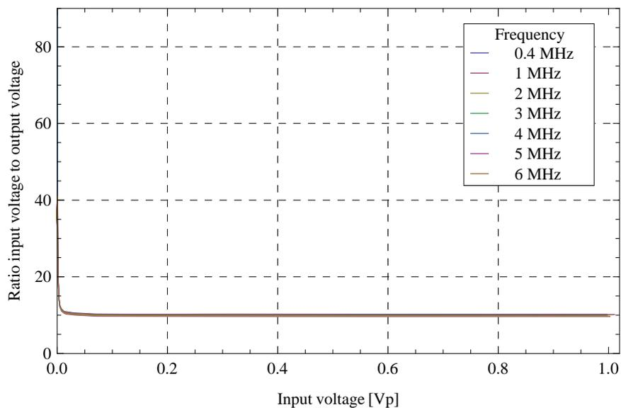
Figure 6.7: *Ratio of input to output signal for the ADC1 channel as a function of input voltage.*
