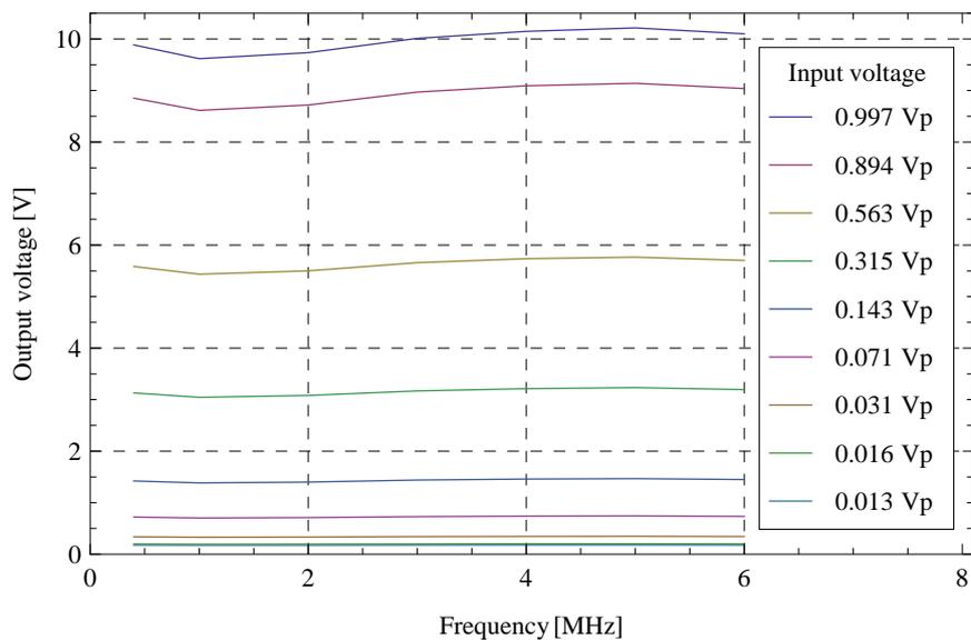
Figure 6.10: *Frequency dependency of ADC2 channel: Output voltage over frequency at several input voltages.*
