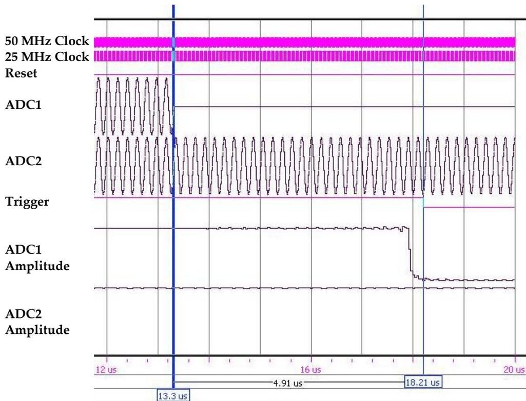
Figure 5.5: *Simulation of detector framework and arc detector core with triggering: From top to bottom the signals of the 50 MHz clock, the 25 MHz clock, the reset, the ADC1, the ADC2, the trigger, the ADC1 amplitude and the ADC2 amplitude are plotted. The blue vertical lines are indicating cursor positions.*
