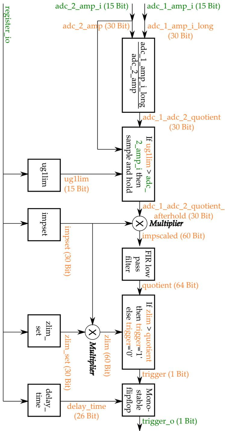
Figure 5.3: Schematic of the arc detector core: Ports are illustrated in green, signals in orange.
