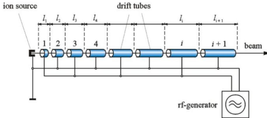
Figure 1.1: *Principle of the Wideroe linear accelerator. On the left hand side particles are emitted by an ion source. RF voltage is applied to the drift tubes, which have an increasing length. The particles are accelerated towards the right hand side.*
