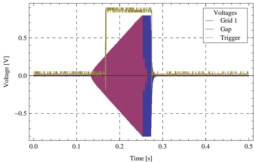
Figure 7.7: Measurement of the trigger signal (divided by 5 for better visibility), the grid-1 voltage, and the gap voltage in a realistic acceleration cycle producing an electric arc.
