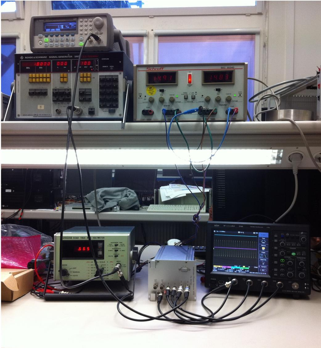
Figure 6.1: *Picture of the Test Setup: On the left hand side of the shelf two arbitrary waveform generator are located. In the right hand side of the shelf there is the voltage supply for the arc detector. On the left hand side on the table is the true RMS voltmeter, in the middle is the arc detector and on the right hand side is the oscilloscope located.*
