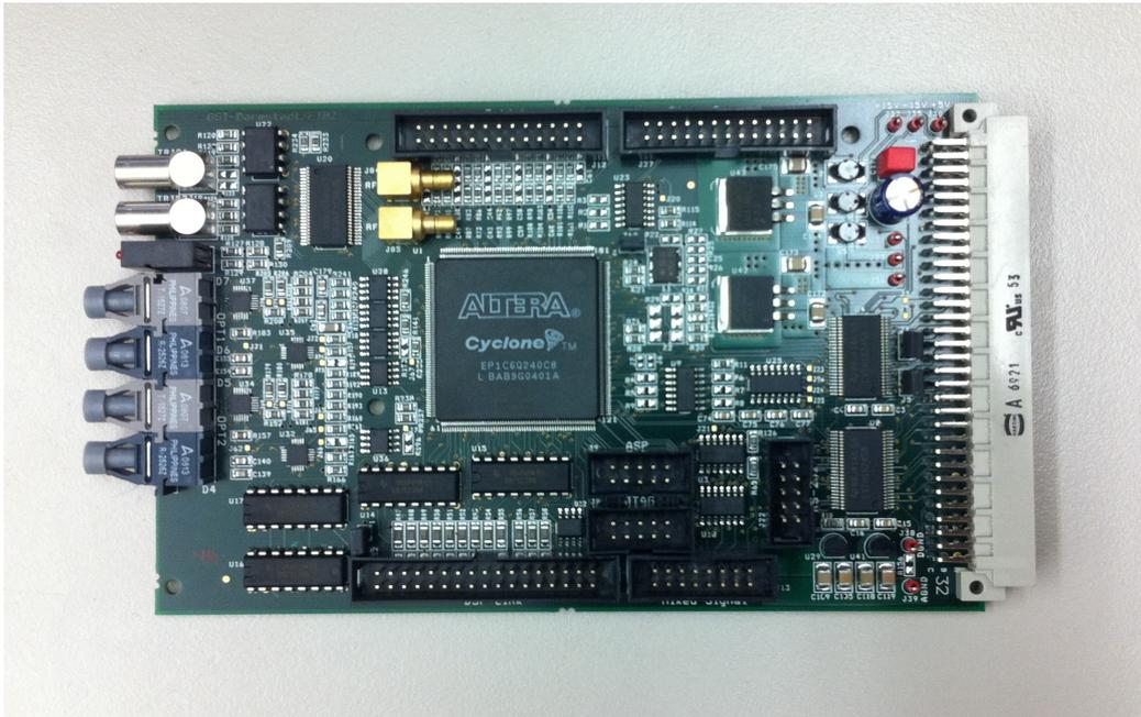
Figure 2.2: *Picture of the FIB (FPGA Interface Board). On the left hand side two LEMO plugs, four LED for displaying a status code, and four optical I/Os. In the center a Cyclone FPGA by Altera. On top and bottom there are several interfaces, see 2.1 for a list. On the right hand side the interface for connecting the FIB to the backplane.*
