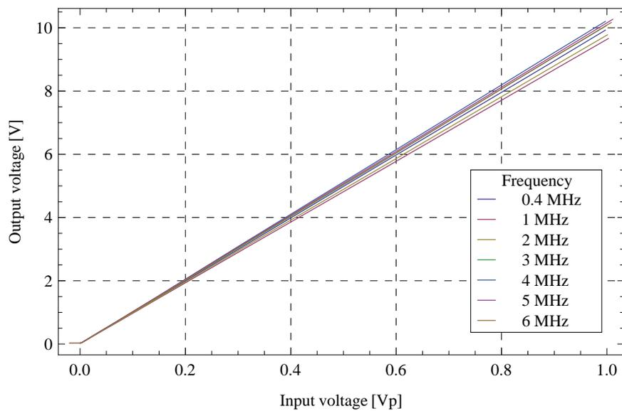
Figure 6.5: *Linearity of ADC1 channel: Output voltage over input voltage measured at several frequencies.*
