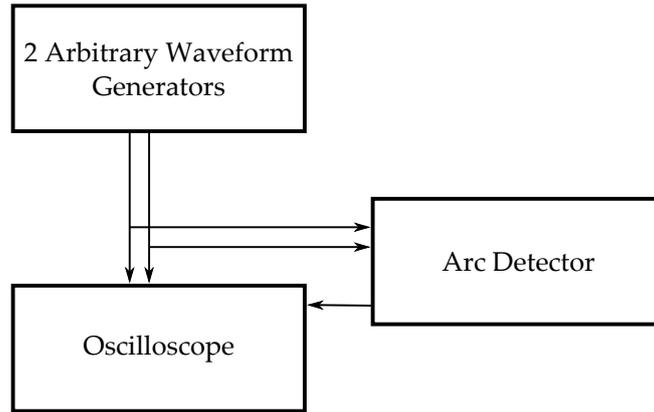
Figure 6.14: *Schematic of the test setup for measuring the characteristics of triggering: Two RF signals generated by arbitrary waveform generators are detected by the oscilloscope and the arc detector. At the same time the trigger output signal of the arc detector is measured by the oscilloscope.*
