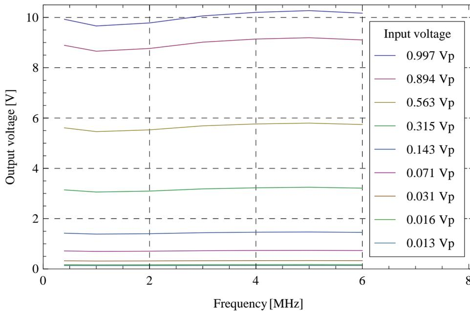
Figure 6.9: *Frequency dependency of ADC1 channel: Output voltage over frequency at several input voltages.*
