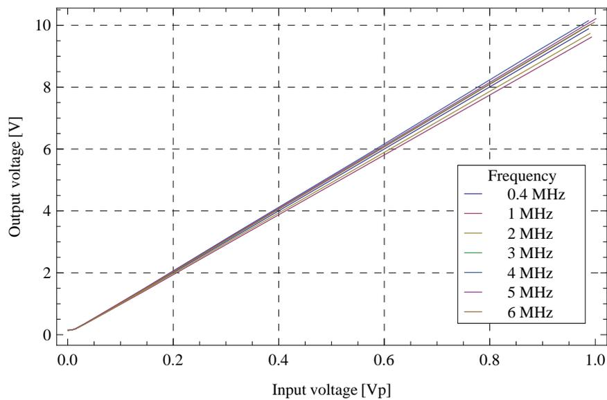
Figure 6.6: *Linearity of ADC2 channel: Output voltage over input voltage measured at several frequencies.*
