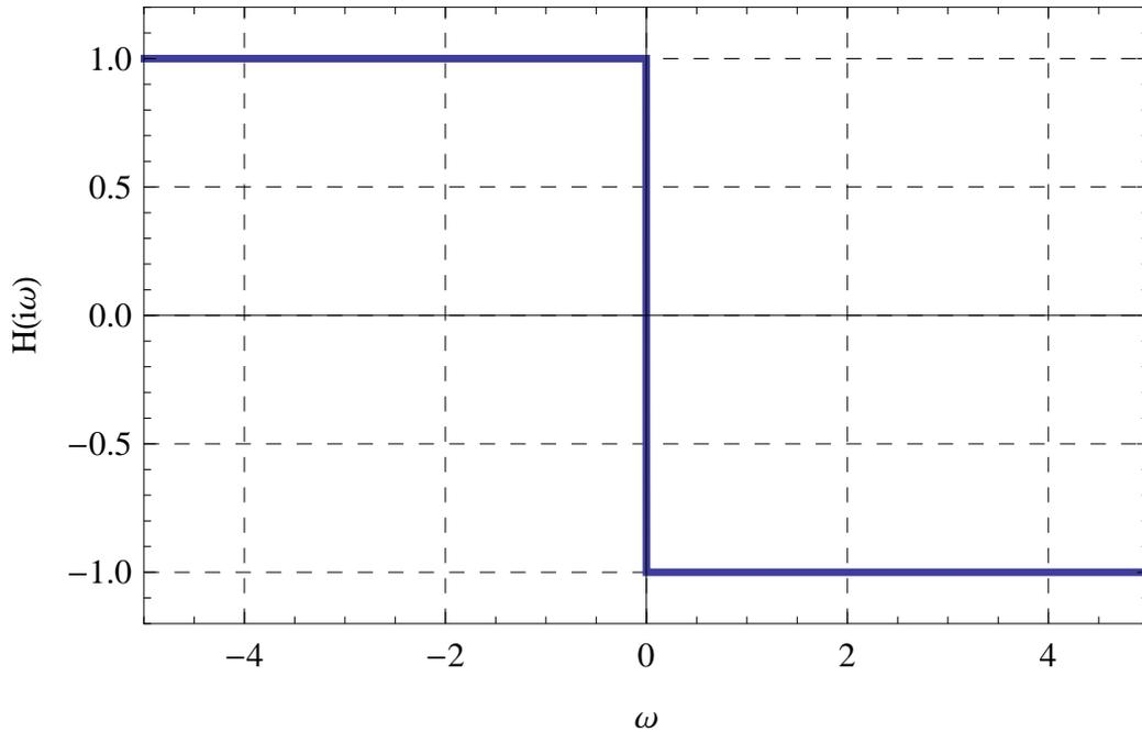
Figure 4.1: *Plot of the frequency response of the Hilbert transfer function.*
