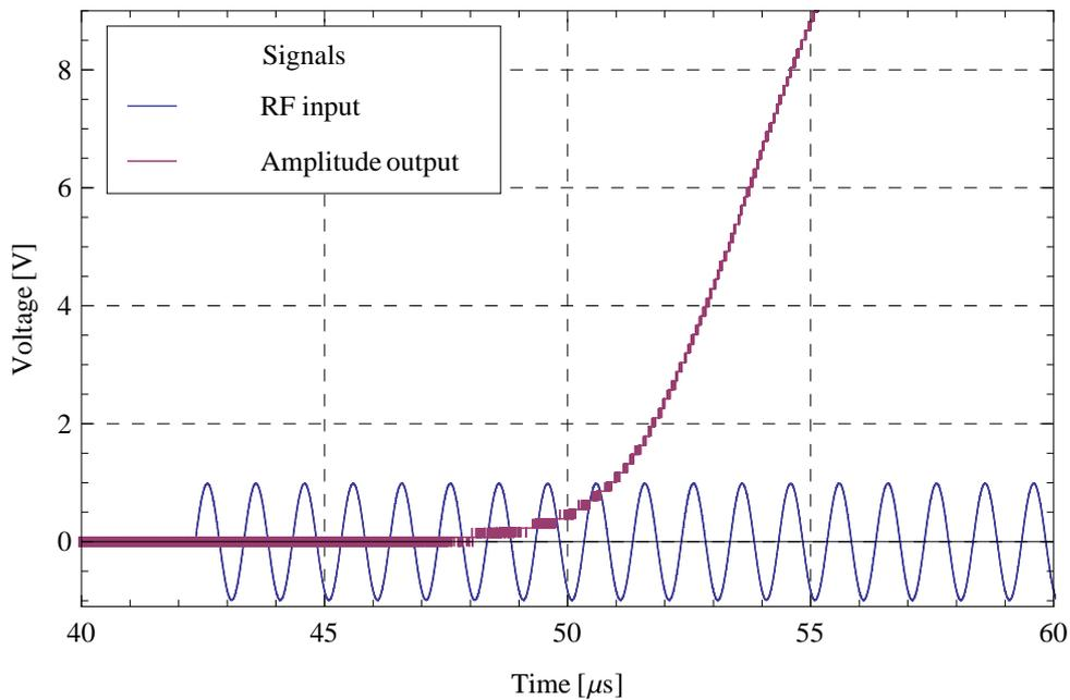
Figure 6.13: *Measurement of the amplitude response time for the example of the ADC1 Channel: The output voltage is displayed as a function of time.*
