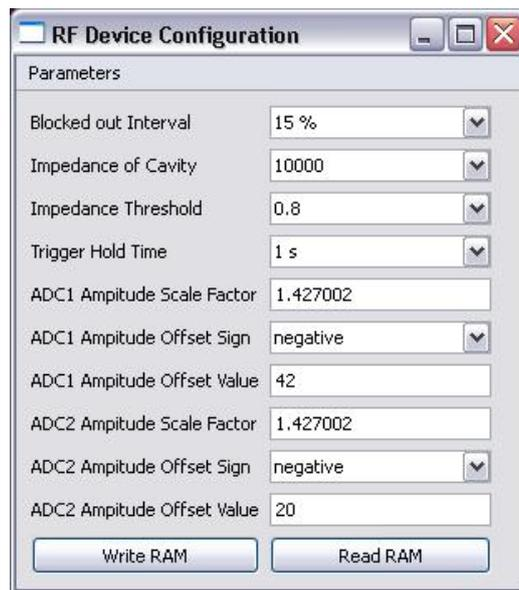
Figure 5.7: *RFDevConf Arc Detector Configuration Menu* consisting of drop-down menus for the blocked-out interval, the impedance of the cavity, the impedance threshold, and the trigger hold time as well as input boxes for the ADC1 and ADC2 amplitude scale factor and the ADC1 and ADC2 offset value with drop down menus to set the respective sign. Below this there are two buttons for reading and writing the RAM.
