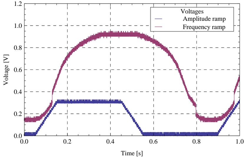
Figure 7.5: *Measurement of the frequency and amplitude ramp set signals.*
