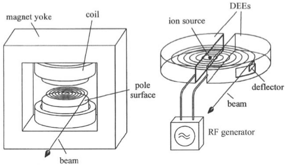
Figure 1.2: *Principle of the cyclotron: On the left hand side a principle of the outer part of the cyclotron shown including the magnet yoke and the coil, which are used for producing a homogeneous magnetic field. On the right hand side there are two D-shaped metal chambers that are connected to a RF generator. Near the center of the chambers the ion source is located. The right chamber has got an deflector for extracting the beam.*
