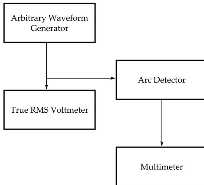
Figure 6.2: *Schematic of the test setup for measurements of characteristics of amplitude detection: The RF signal generated by the arbitrary waveform generator is detected by a true RMS voltmeter and the arc detector. The amplitude signal generated by the arc detector is measured by a multimeter.*
