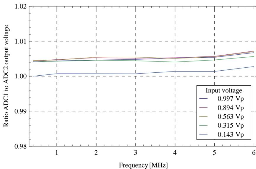
Figure 6.11: *Ratio of output voltages from the ADC1 and ADC2 channels as a function of frequency for several input voltages.*
