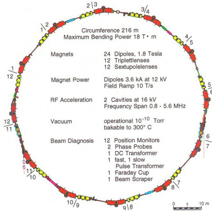
Figure 1.3: Schematic of heavy-ion synchrotron SIS-18. The dipole bending magnets are illustrated in red, the quadrupole focusing magnets in yellow, and the acceleration cavities in blue. The SIS-18 is divided in twelve similar cells.
