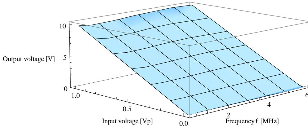
Figure 6.3: *Measured values of ADC1 channel: Plotted is the output voltage as a function of the voltage and the frequency.*
