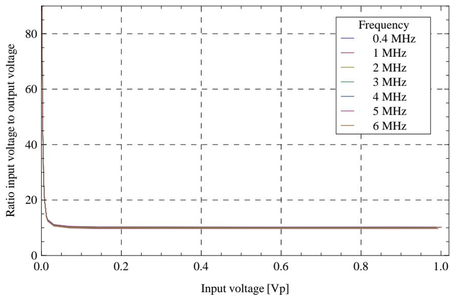
Figure 6.8: *Ratio of input to output signal for the ADC2 channel as a function of input voltage.*
