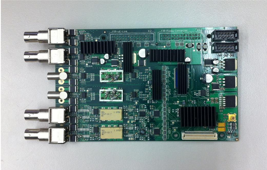
Figure 2.4: *Picture of the ADC/DAC FAB (FIB Adapter Board). On the left hand side from top to bottom two BNC plugs for monitoring the ADC input signals, two LEMO plugs for output, and two BNC plugs for AC input. Top right two programming interfaces for ASP and JTAG. Bottom right a FPGA Cyclone III covered by a cooler.*
