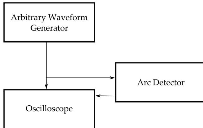
Figure 6.12: Schematic drawing of the test setup for measuring the rise time for the amplitude detection: The RF signal generated by the arbitrary waveform generator is detected by the oscilloscope and the arc detector. The amplitude output signal of the arc detector is also measured by the oscilloscope.
